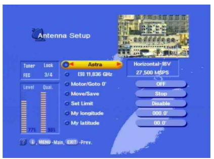
The first line is used to specify the satellite and the second line to specify the transponder.
